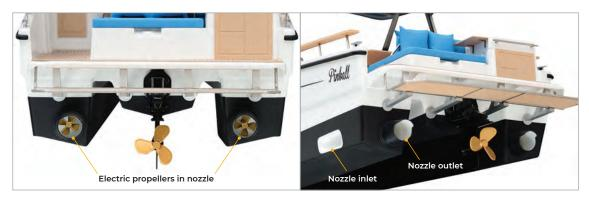
Nozzles are 30 cm diameter tubes, profiled to accelerate water flow forward. Range is 2 hours at 4 knts and 1h20 at 5 knts.
