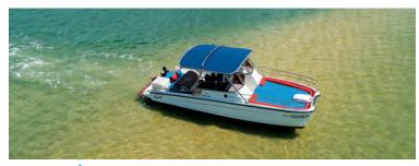
> When operating in Electric, engine is off, sterndrive is up and electric propellers are secured in nozzles. This is better for swimmers safety and you can go gently in shallow water without the worry of damaging propellers.
